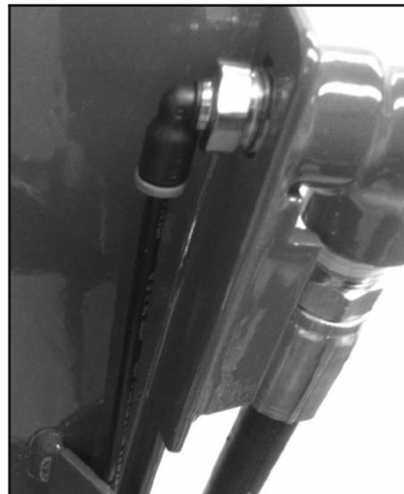
4. Route the internal air hose into the side groove of the repair stand and have it exit at the pump mounting location (three circular holes). Connect the non-threaded elbow fitting to the hose by pressing it in until it bottoms out.
